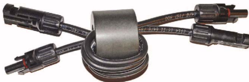
Figure 5 — Three bifilar turns of #10 PV wire on Fair-Rite 2631626202 core with MC4 connectors installed.
